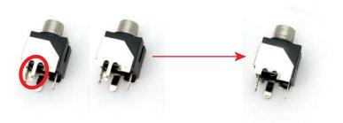
STEP 5: Place and all parts on the pcb, notice the difference between the jacks. Once placed allign with the frontpanel and tighten all the nuts.
