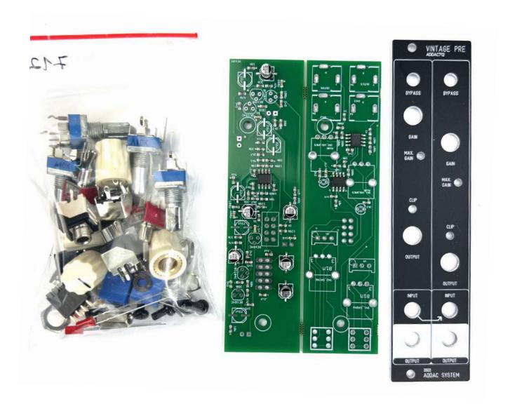
STEP 1: Grab the pcb, gently brake it apart and trim the excess with a cutting plier.
