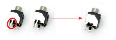
STEP 12: Place the remaining parts on the pcb, allign the front panel and tighten the jacks and pots' nuts.
