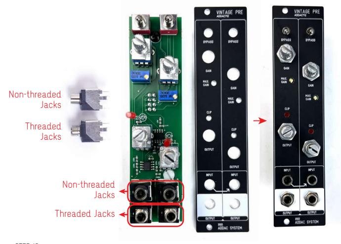
STEP 13: Adjust the height of the pcb keeping it parallel to the front panel and proceed to solder all parts.
