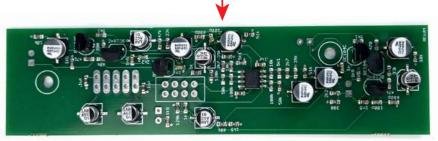
STEP 4: Locate the two 120uf capacitors, straighten their legs as shown below.
