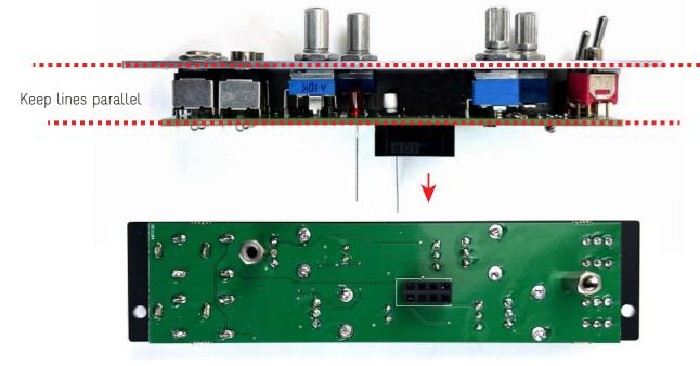
Finish it by placing the knobs and you've finished the assembly process!
