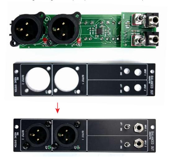
Finish it by fixing the XLR connectors with the screws and soldering the connectors.
