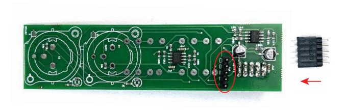
STEP 4: Allign both pcbs and solder the pinheader to the top pcb  $\,$
