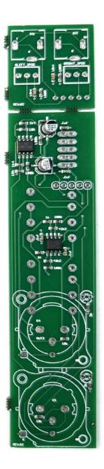
STEP 1: Grab the pcb, gently brake it apart and trim the excess with a cutting plier.
