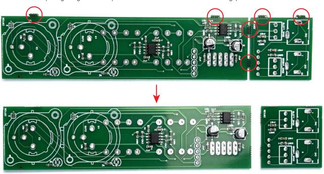
STEP 2: Place and solder the 2x5 boxed pinheader. Notice the indent orientation.
