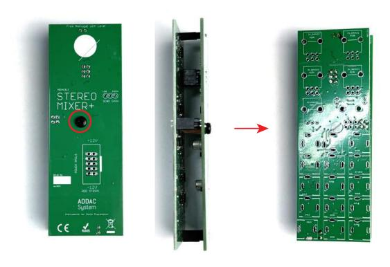
STEP 5: Next place and solder the remaining pinheader and boxed header .Notice the orientation of the boxed header.
