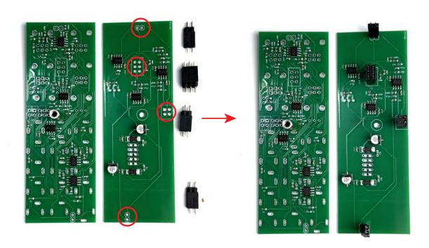
STEP 4: Proceed by placing the back screw to hold the pinheaders in place and solder them to both pcbs
