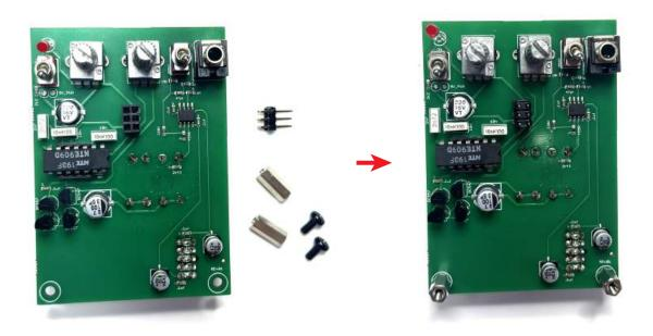
STEP 9: Place the frontpanel and screw it in place. Then solder all parts.
