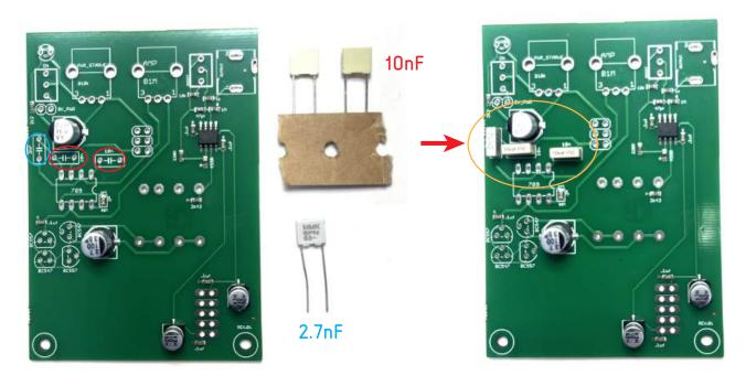
STEP 2: Proceed by placing and solder the transistors, notice there are 2 types.
