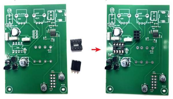
STEP 4: Next place the NTE909D IC, notice the orientation of the IC and how the legs are placed in the socket.
