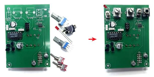
STEP 8: Place the 2 bottom spacers and fit the 3x2 male pinheader into the female.
