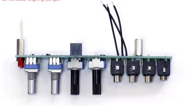
STEP 10: Place the front panel and tighten the 3 nuts Make sure the pcb is parallel to the frontpanel
