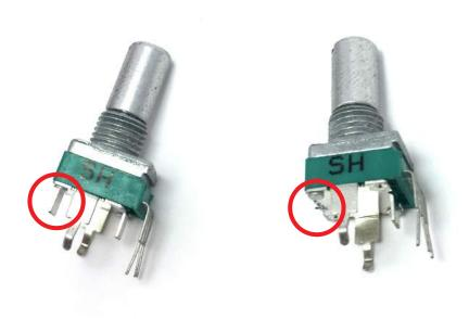
STEP 5: Locate the 10k trimmer potentiometer and use some pliers to straighten the side pieces.
