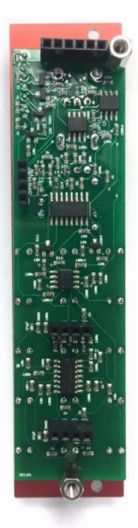
STEP 8: Locate the bottom pcb and proceed by placing and solder the 2x5 boxed header.
