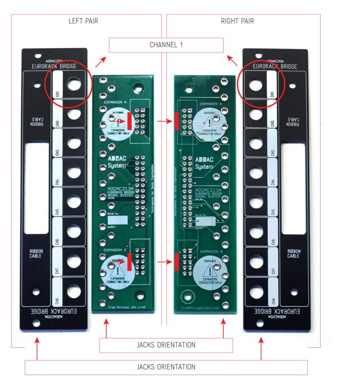
We'll now assemble the Right Module, you can follow the same principles to assemble the Left module.
